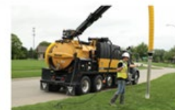
PTO DRIVE SYSTEM. A side PTO drive system allows the vac to keep running while moving the truck between holes, rather than requiring full machine shutdown for each move.
