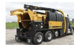
CAM-OVER REAR DOOR. The highly reliable cam-over design provides a 360-degree positive seal, with no additional clamping and no in-tank moving parts.
